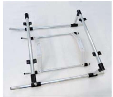
The Lama u/c is much bigger than the donor skid set; note the saw cuts in the 'L' moulds...
