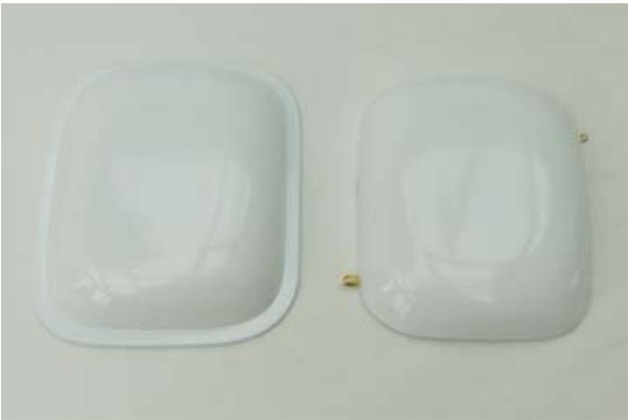
On the left is a tank cover as supplied, on the right is my modified version complete with brass fixing brackets that are glued to the inside
