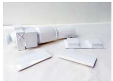
Dummy turbine with the tail stabilisers
