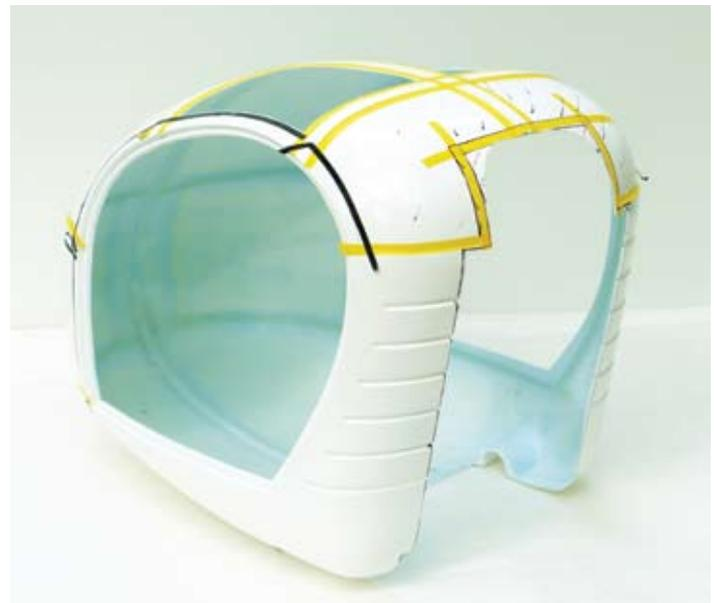
*The back was cut out using John White's measurements; I didn't cut out all the windows as I wanted it to stay rigid, I need not have worried as you can see the reinforcing strips round the windows and doors*
