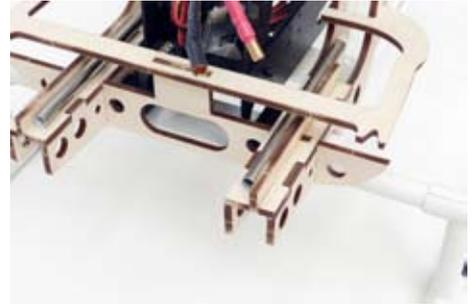
*The canopy tubes fit over these and are glued to the wood*
