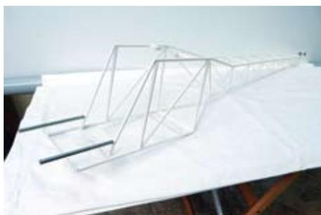
Vario supply the lattice tail 'bare', mine has been powder coated
