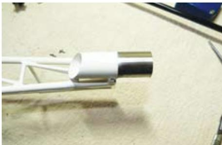
This is the 20 mm tube to take the Vario tail gearbox, but the T-Rex boom is 21.5 mm
