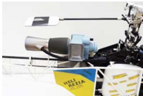
*The dummy turbine is supported with short tubes*
