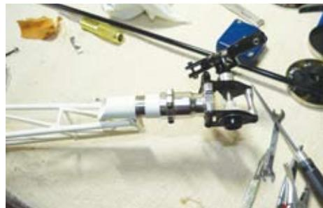
Here I have painted a short off-cut of the Align boom that slides over the Vario tube
