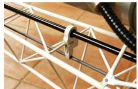
Tail tube support with the pitch rod support below
